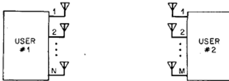
Fig. 6. Radio system consisting of two users, one with M antennas and the other with N antennas.
